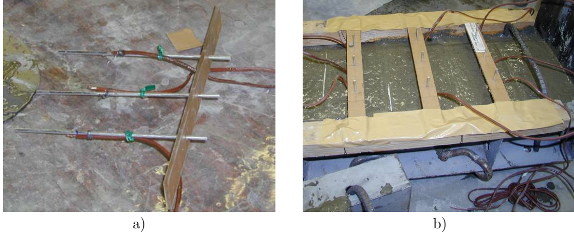
Figure 2.53: a) Setup for temperature sensors; b) appearance after casting
