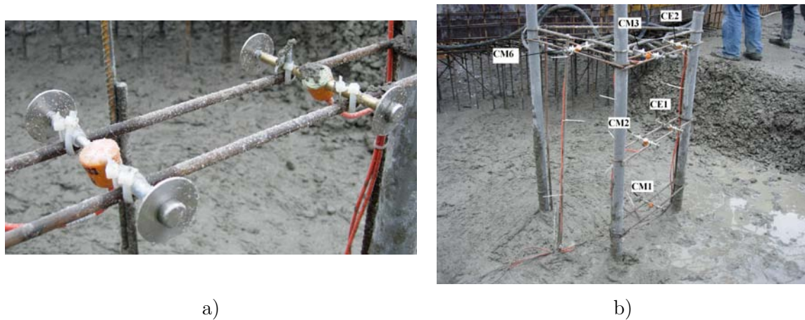
Figure 6.33: a) Fixation of the strain gages; b) photo of sensors positioned in the tubes
