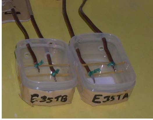
Figure 4.22: Forms and thermocouples used for the evaporative cooling experiment
