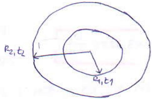
$$\phi = \frac{t_1 - t_2}{\frac{1}{2\pi} \cdot \frac{1}{\lambda} \left( \frac{1}{R_1} - \frac{1}{R_2} \right)}$$
