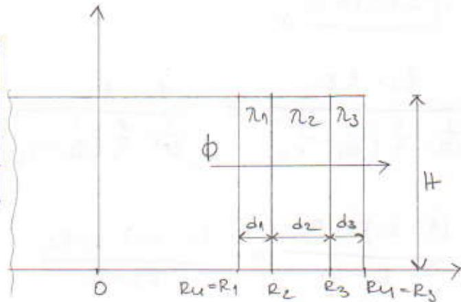
$$\Phi = \frac{\Delta t}{\frac{1}{2\pi H} \left( \frac{1}{\alpha_1 R_1} + \sum_{i=1}^3 \frac{1}{\lambda_i} \ln\left(\frac{R_{i+1}}{R_i}\right) + \frac{1}{\alpha_2 R_4} \right)} = \frac{20 \cdot 2\pi \cdot 10}{\frac{1}{7,69 \cdot 3,5} + \frac{1}{1,4} \ln\left(\frac{3,515}{3,5}\right) + \frac{1}{2,33} \left(\frac{3,915}{3,515}\right) + \frac{1}{1,4} \left(\frac{3,945}{3,915}\right) + \frac{1}{25 \cdot 3,945}}$$
