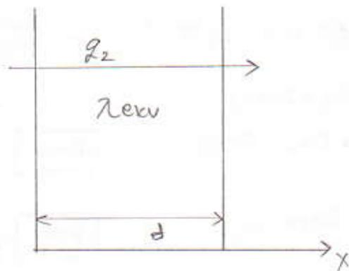
$$q_1 = \frac{t_1 - t_2}{\sum R_i} = \frac{t_1 - t_2}{\frac{d_1}{\lambda_1} + \frac{d_2}{\lambda_2} + \dots + \frac{d_n}{\lambda_n}}$$
