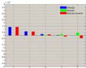
Fig. 4 Diagram of potential and kinetic energy growth rate distributions and their mutual difference for modified and original cantilever beam [J].
