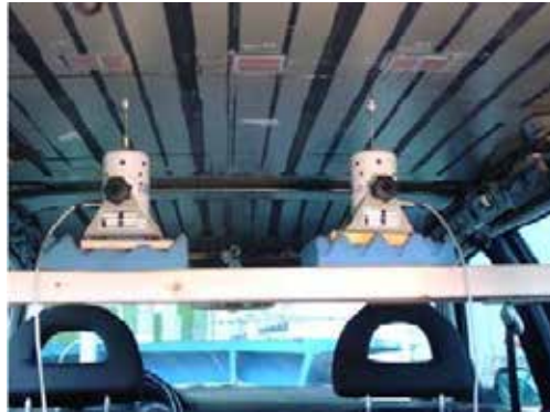
Figure 19: Passenger compartment and inner surface of the car roof with attached piezoelectric patches and exciting shakers
